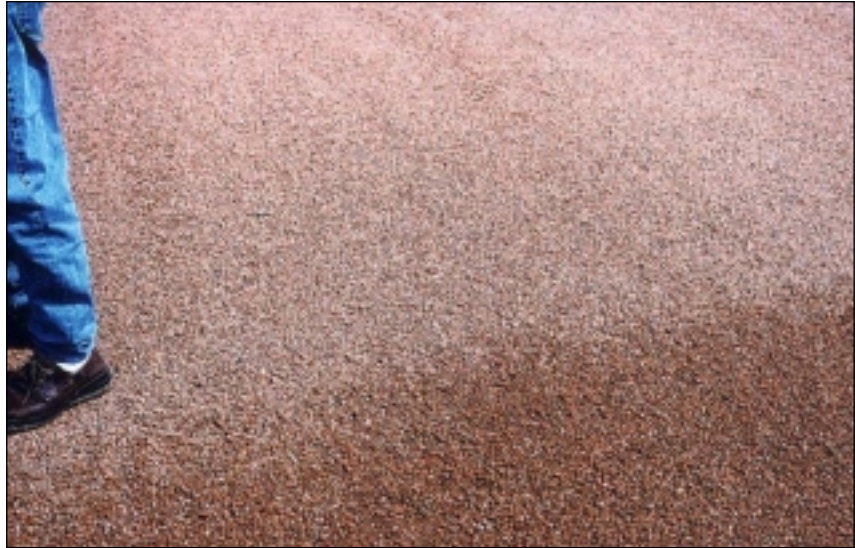
Surface moisture on just-laid LITE-WATE at bottom is darker than that above which has lost some of its moisture after 1 hour.
