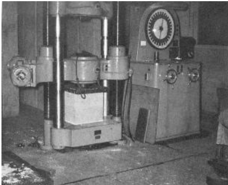
Figure 10.23. Test setup for 2-high prisms
