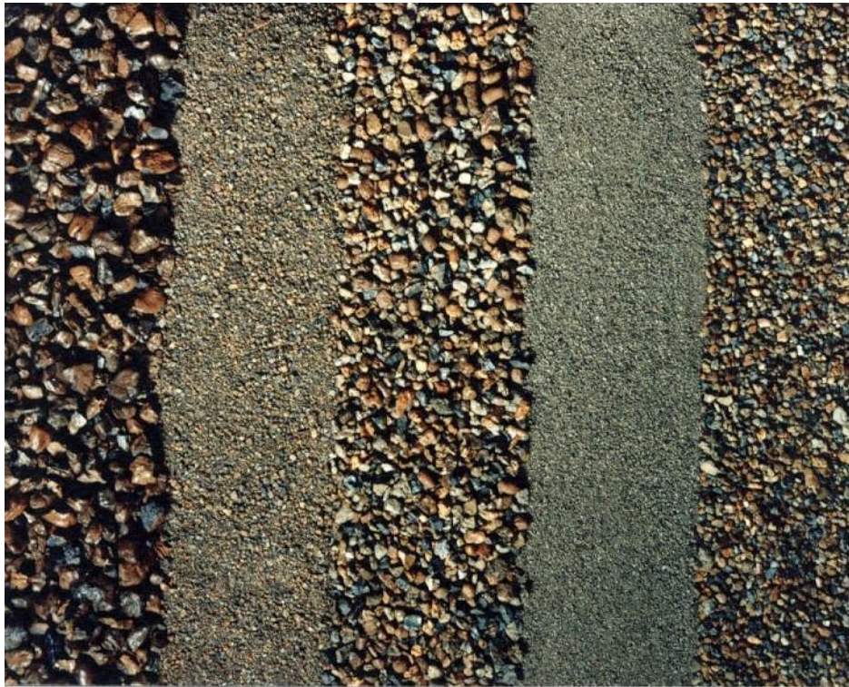
3/4 inch (19mm) No. 4 & Finer (4.75mm) 1/2 inch (12.5mm) No. 8 & Finer (2.36mm) 3/8 inch (9.5mm)
