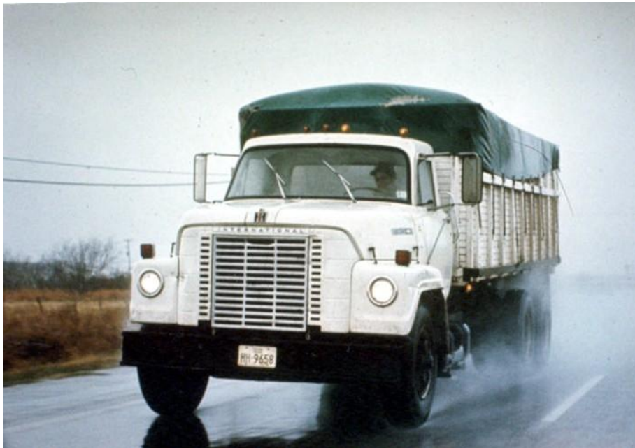
Figure 14.16 Regular hot-mix asphalt surface with hazardous truck spray and splash
