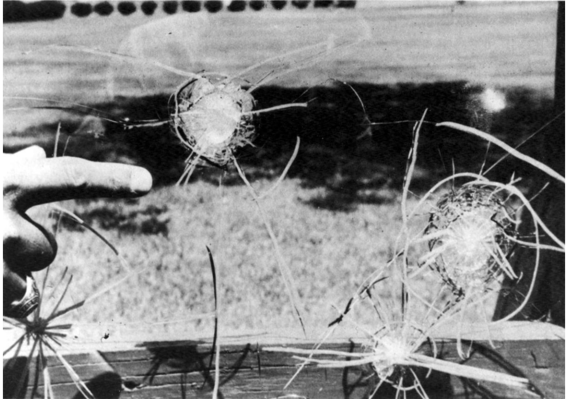
Figure 14.7 Windshield damage with normalweight cover aggregate (trap rock, crushed limestone, gravel, blast furnace slag, etc.)
