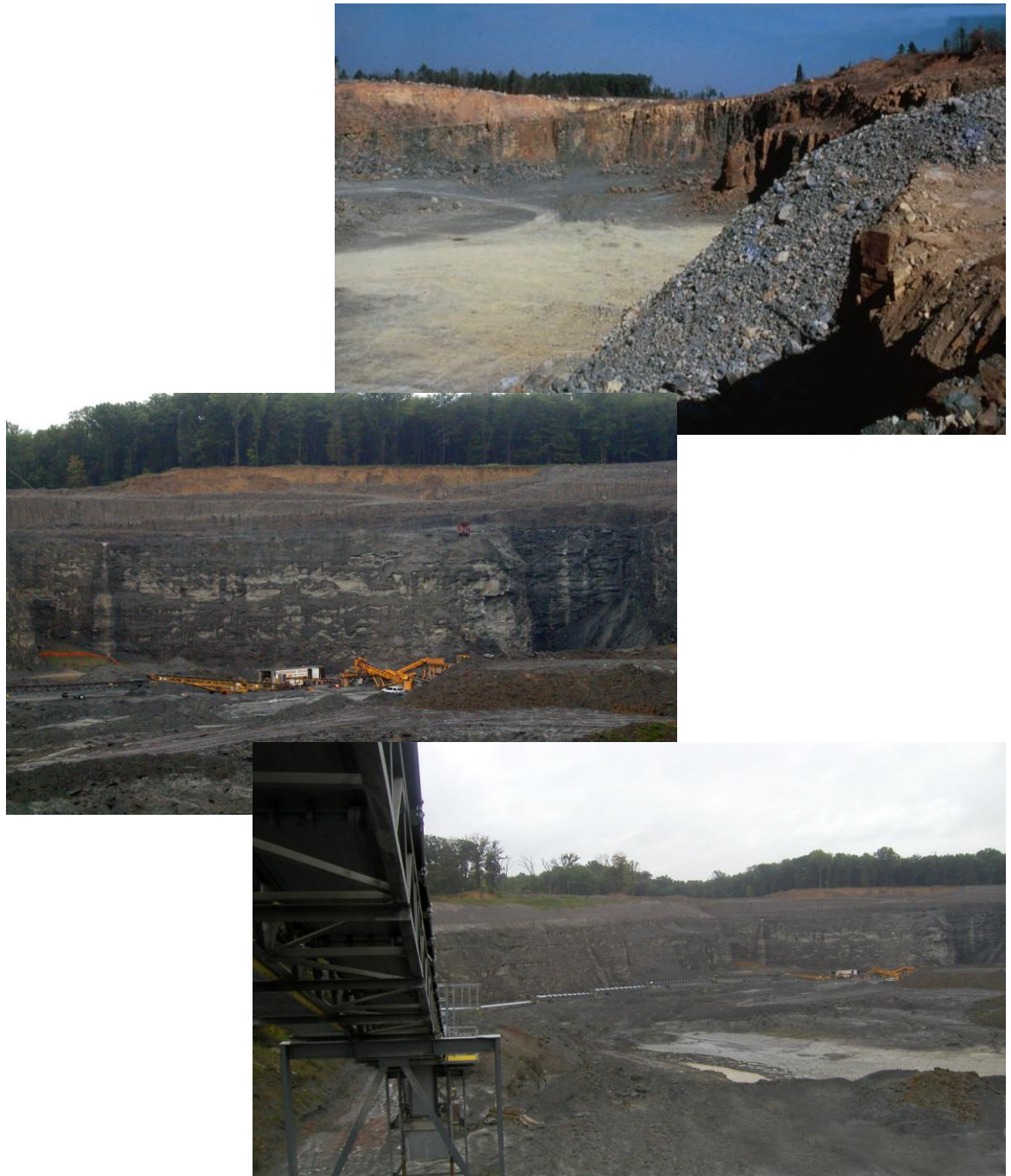
Figure 2.4. ESCS is produced from deposits of shale's, clays, and slates. These minerals are principally composed of silica and alumina, similar to those used in brick and other ceramics known to be extremely durable. From the quarry (deposit) the raw material is taken to the preliminary crushing/screening plant, and then expanded in a rotary kiln.
