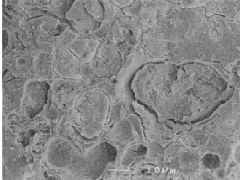
Figure 8.4. Concrete with a precipitation of alkali-rich material in the pores of lightweight aggregate (Boyd 1998).
