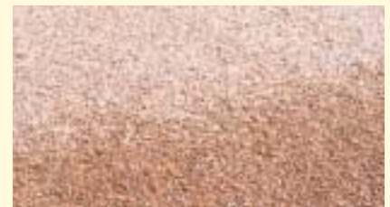
Surface moisture on just-laid Lite-Wate, one-hour old, above, has lost its surface moisture.
