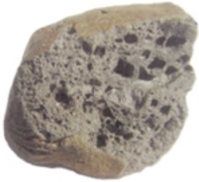
SOILMatrix particle showing interior voids
