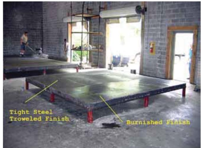
Fig. 2: Finished concrete surfaces from Study 1
