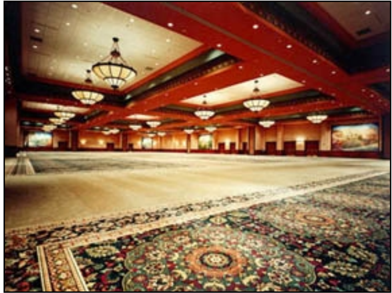
Clear-span ballroom and convention space made possible by long-span lightweight concrete double tees (Courtesy: John Q. Hammons Hotels, Inc.)
