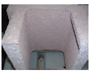
Lightweight CMU with current generation integral water repellant admixture after water penetration test
