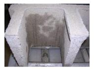
Lightweight CMU with first generation integral water repellant admixture after water penetration test
