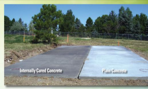
Both slabs installed within minutes of each other. No conventional curing on either slab. Photograph taken 24 hours later.
