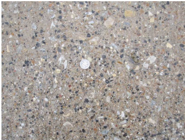
Figure 31. Close-up view of ICC pavement surface at Windsor Park subdivision. The black specs in the surface are the larger pieces of LWA.
