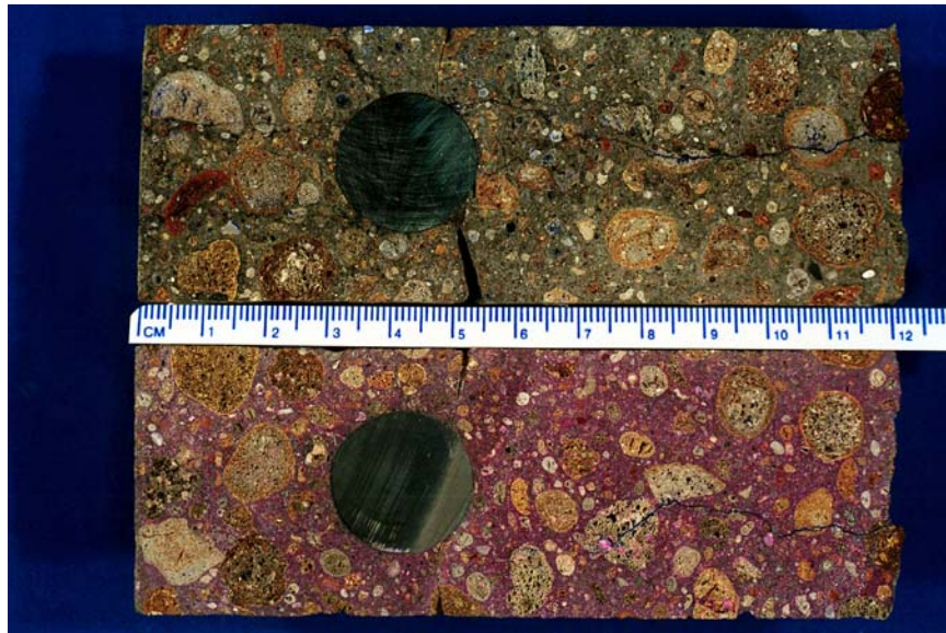
Fig. 5 Longitudinally cross sections of a core drilled over a diagonal crack along the hull of the Armand Concidere shows no corrosion of steel and minimal carbonation of paste. The lower section was treated with phenolphthalein.
