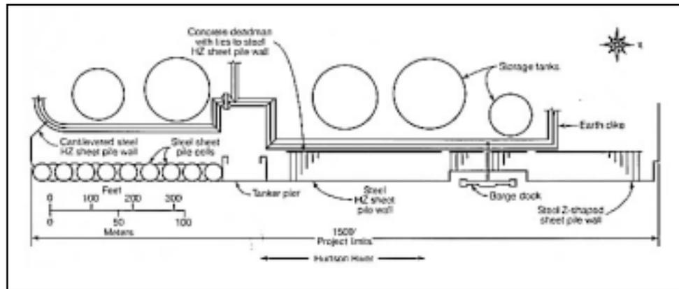
Fig. 2 Overview of Marine Terminal Modifications
