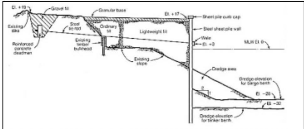
Fig. 1 Cross-section at Sheet Pile Wall
