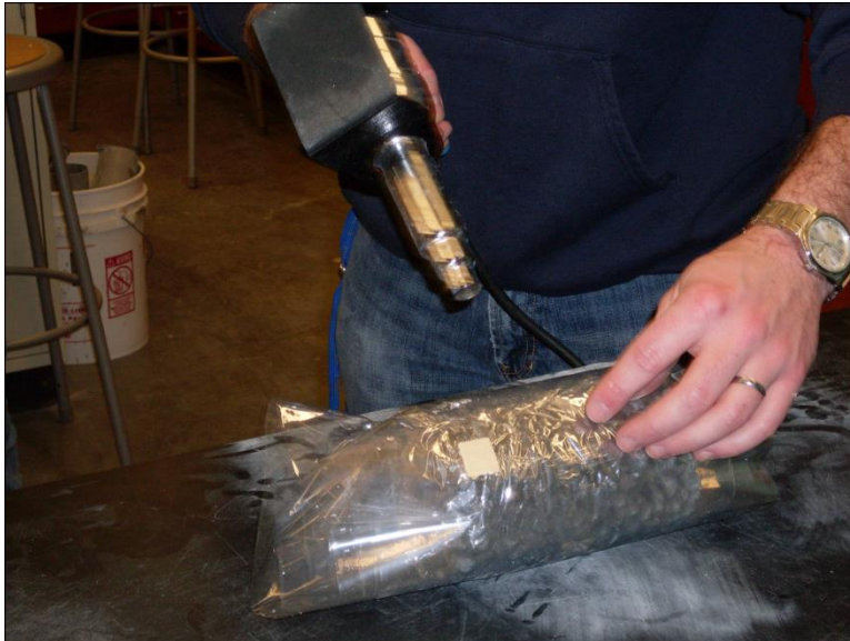
Fig. 1. Sealing Samples in Heat Shrink Tubing
