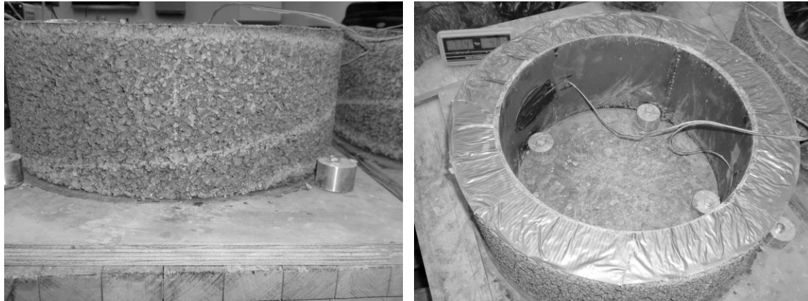
Fig. 5. Ring Shrinkage Testing on Pervious Concrete
