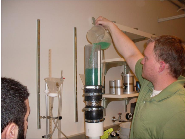
Fig. 2. Permeameter Testing (Green Water Shown for Contrast)
