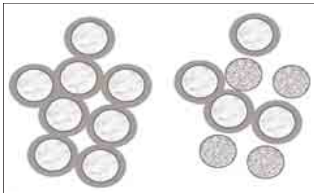
Figure 7. Comparison of model mortars with normal weight sand particles only (left) with their surrounding ITZs and with a 50:50 blend (volume basis) of sand and LWA (right). Both the volume fraction of ITZ (grey) paste and its percolation (top to bottom) are significantly reduced by the incorporation of the LWA.
