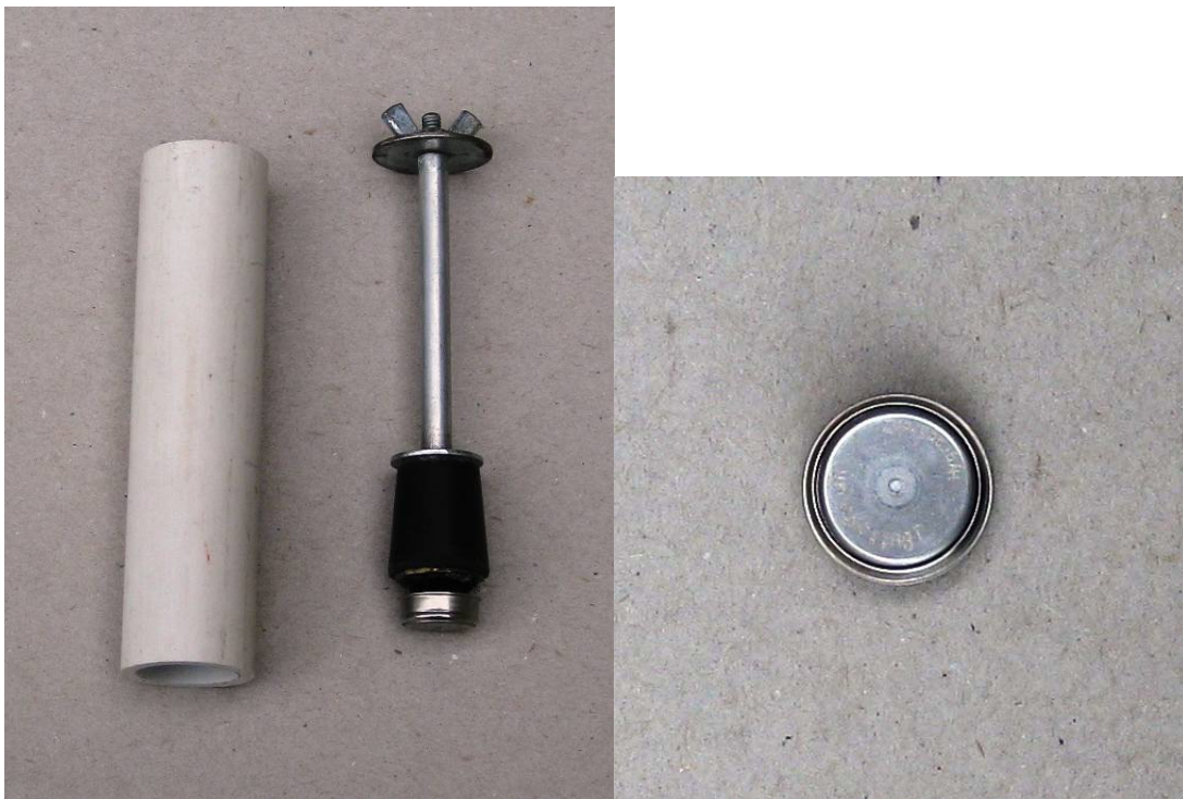
Figure 2. Humidity/Temperature Probe and Assembly. The rubber stopper is compressed by turning the thumbscrew to seal the probe near the base of the pipe. The pipe has an inside diameter of 1 in.
