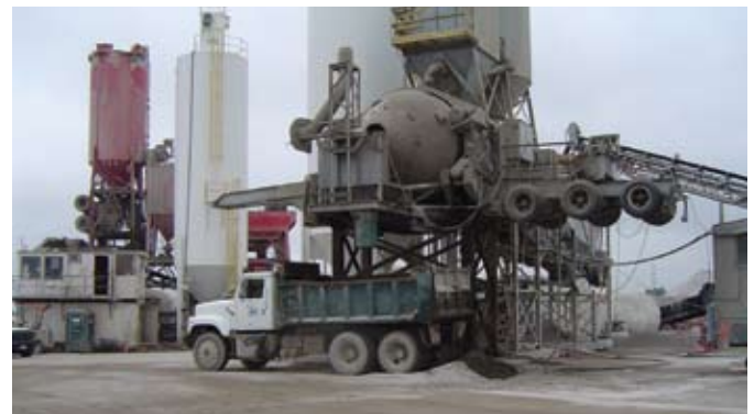
Fig. 3: Double central-mix batch plant at the Union Pacific Intermodal facility in Hutchins, TX
