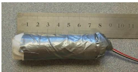
Figure 5-5- Encapsulated relative humidity sensor before embedment in concrete
