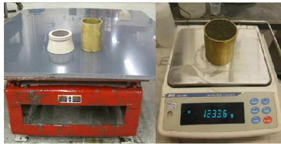
Figure 3-12- Packing density test setup
