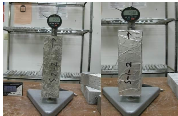
Figure 3-21- Shrinkage measurement of unsealed (left) and sealed specimens (right)
