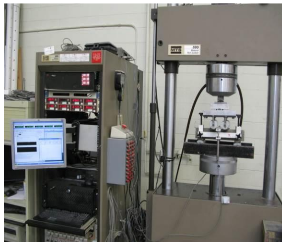
Figure 3-16- Test setup for flexural toughness measurement of FRC beams
