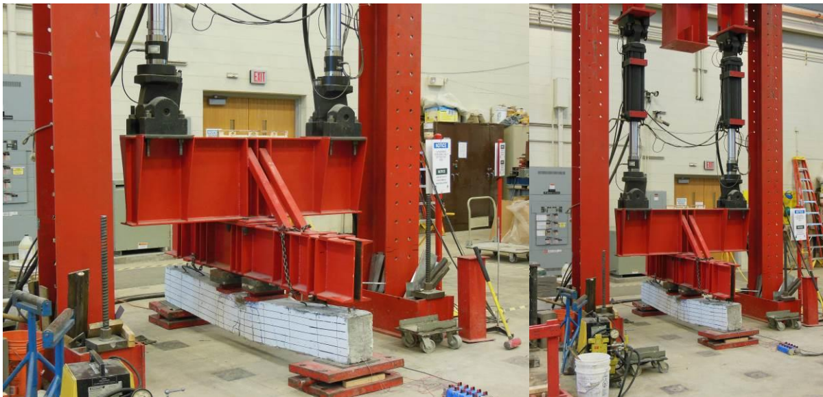
Figure 5-14- Beam flexural test setup
