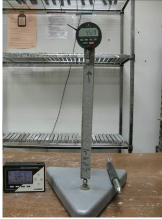
Figure 3-15- Drying shrinkage measurement of mortar
