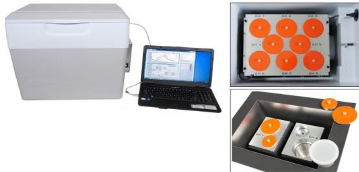
Figure 3-9- Isothermal calorimetry used for hydration kinetics of mortar
