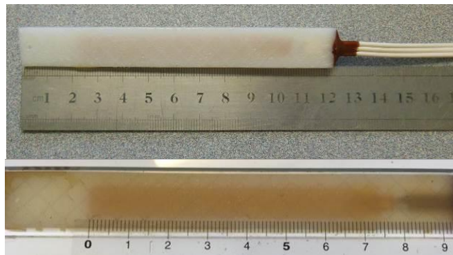
Figure 5-2- Embedded strain gauge for monitoring shrinkage deformation
