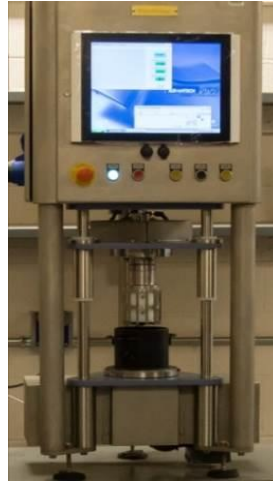
Figure 3-10- Coaxial cylinders rheometer used to determine rheological properties of mortar
