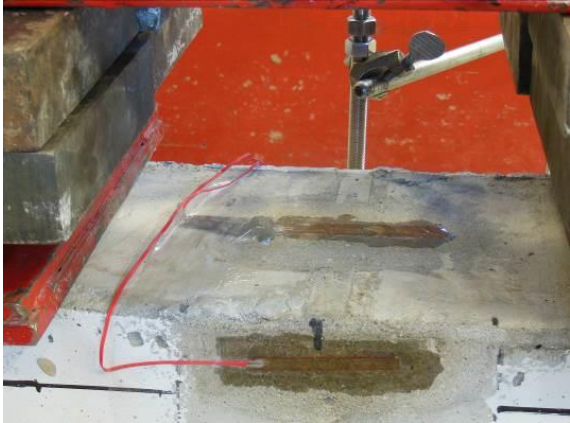
strain gauges on upper surface and lateral side of beam mid-span
