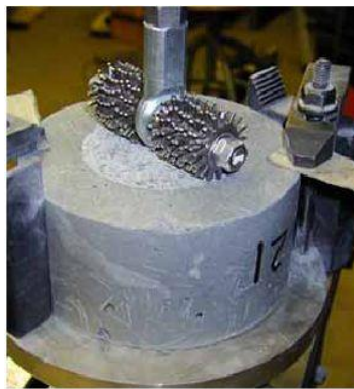
Figure 3-17- Abrasion resistance test setup
