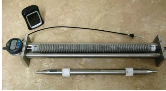
Figure 3-13- Autogenous shrinkage measurement device
