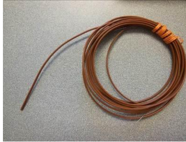
Figure 5-3- Thermocouple used for concrete temperature measurement
