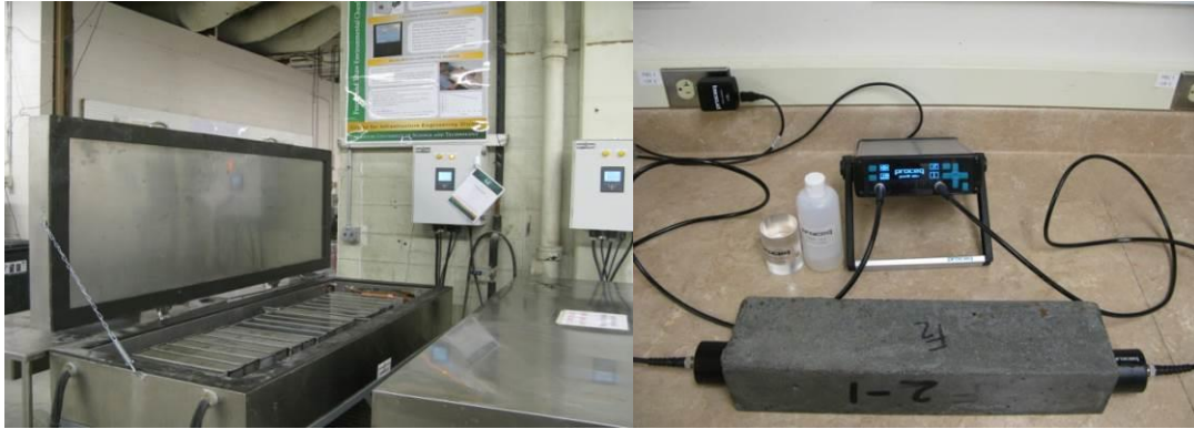
Figure 3-18- Freeze-thaw chamber (left) and ultrasonic velocity instrument (right)
