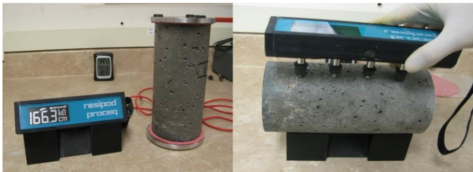
Figure 3-19- Bulk electrical conductivity (left) and surface resistivity (right)
