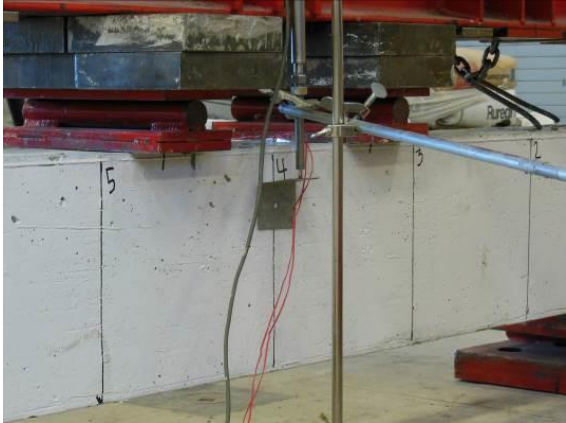
LVDT at mid-span
