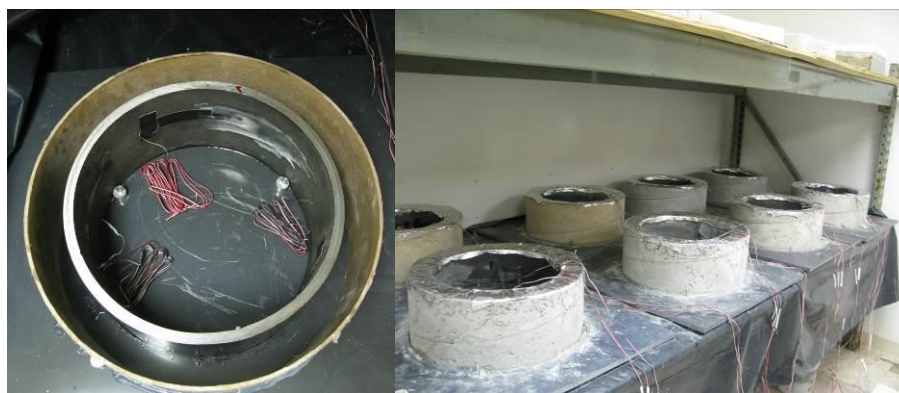
Figure 3-22- Restrained shrinkage ring test setup
